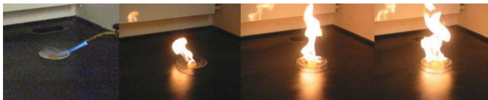
Fig. 2 Ignition test of 1 g of protonated [1-Bu-3-H-im][NO 3 ].
